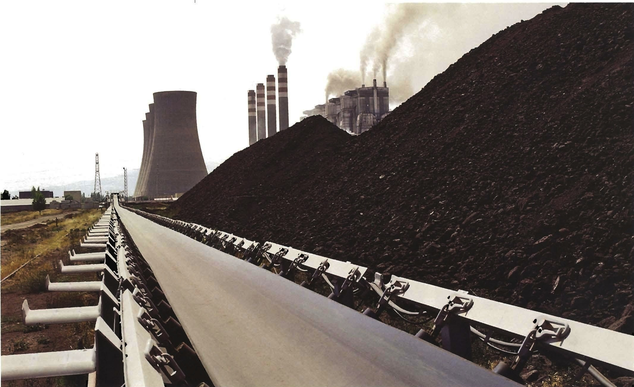
▲ Coal Stock Area's Belt / ST - 2000 / 1600 mm
