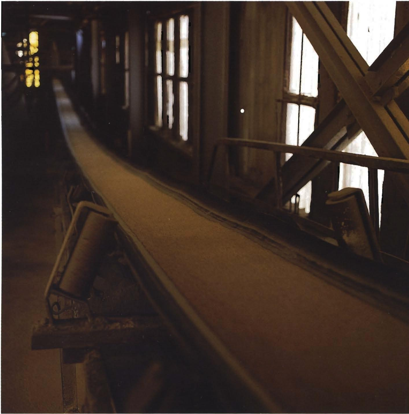
▲ Oily Fertilizer Belt 650 mm/EP 500
